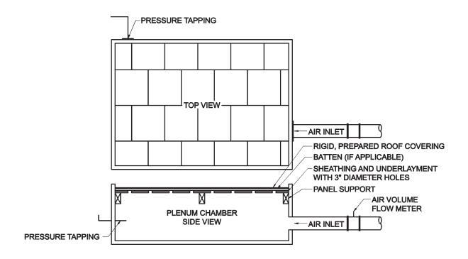
FIGURE 1 AIR PERMEABILITY TEST APPARATUS
